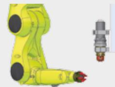
The workpiece carrier system can also move the substrate three-dimensionally. The plasma torch is fixed. It is also possible to coat rotation symmetrical components using suitable clamping device. The plasma torch can also be fitted to the robot arm.
