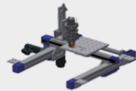
The workpiece carrier system moves the substrate in the X and Y axis. The plasma torch is fixed and can be adjusted manually in the Z level.
